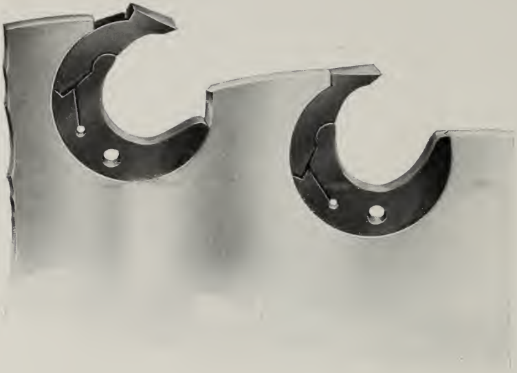
Section of Chisel-Tooth Saw showing how the Bits and Shanks are inserted in the plate.
